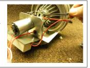
**STEP 9:** Connect the white wire from the LED driver to the red wire from the motor and the long red hook-up wire using a wire nut. Use a wire tie to bundle the wires as shown. Run the wire tie through the hole in the backplate to secure. Carefully insert the entire assembly into the housing. For easier future disassemblies, we recommend applying
