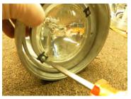
**STEP 4:** Detach gray and red wires from the back of the light housing by removing the small nuts and bolts that secure them to the backplate.
