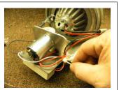
a small amount of anti-seize lubricant to the mating surfaces of the bullet housing and light housing assembly. Reinstall lens, trim ring, and pedestal in reverse order of disassembly.
