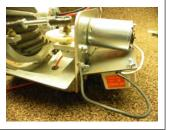
**STEP 8: LED Driver Hook-up:** Connect the **red** wire from the LED Driver to the **red** wire of the LED Module. Connect the **black** wire from the LED Driver to the **black** wire of the LED Module. Use supplied wire nuts for these connections.
