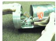
STEP 3: Unscrew and disconnect the two gray wires that are attached to the back of the bulb. From the front of the light housing assembly, remove the two screws and black retaining clips that secure the bulb to the housing. Remove and discard bulb and clips.
